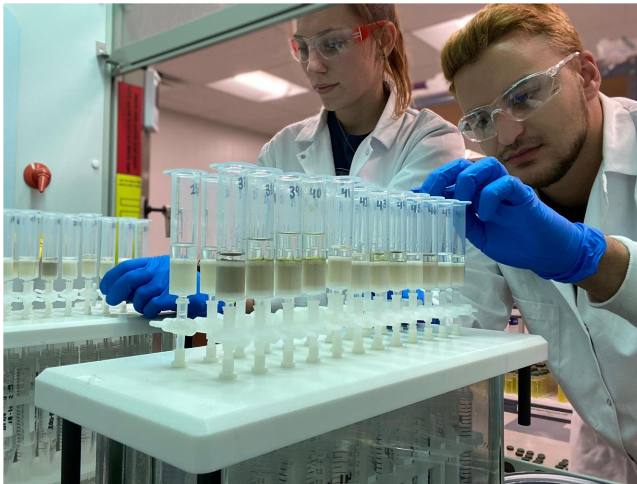
Graduate student Brian Martinez and undergraduate Allison Oldnettle performing solid-phase extraction for PFAS
